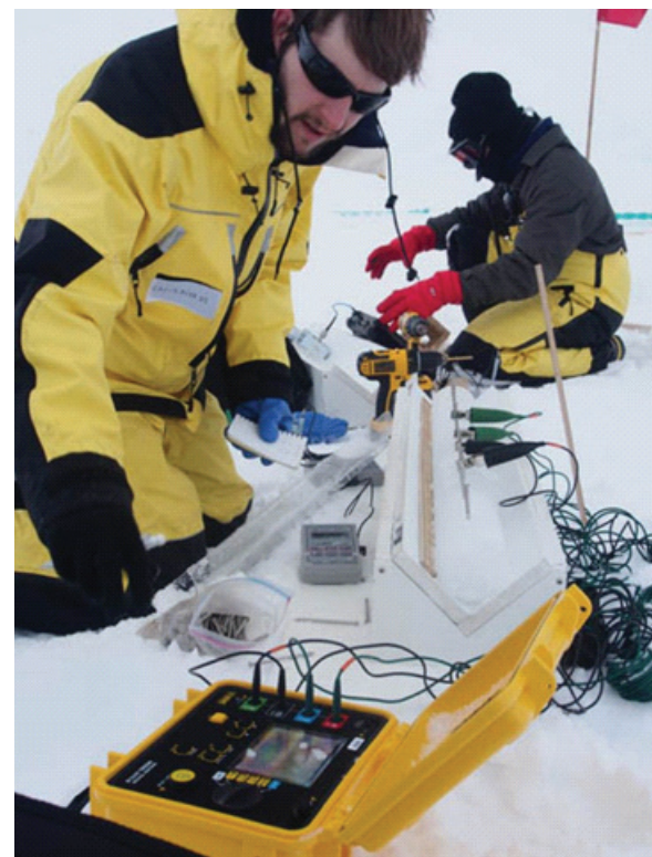
Figure TF6-5: University of Utah mathematics Ph.D. student Christian Sampson measures the electrical conductivity of a sea-ice core during the Sea Ice Physics and Ecosystem eXperiment in 2012. Electrical clamps are attached to nails inserted along the length of the ice core. (© Wendy Pyper/Australian Antarctic Division.)
