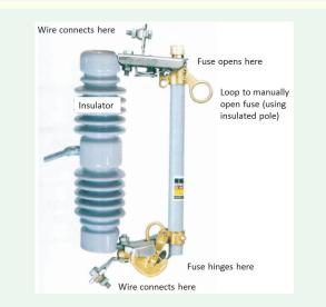
Figure TF26-7: Expulsion fuse cutout for 15 kV–27 kV.
